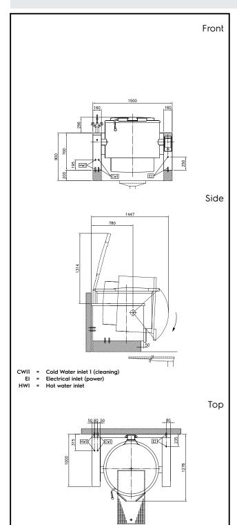
**Electric** Supply voltage: 400 V/3N ph/50/60 Hz Total Watts: 48.2 kW Installation: FS on concrete base;FS on feet;On base;Standing Type of installation: against wall **Key Information:** Working Temperature MIN: 50 °C Working Temperature MAX: 110 °C Vessel (round) diameter: 900 mm Vessel (round) depth: 720 mm
